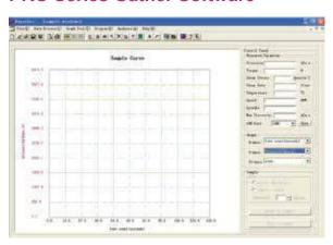
PRO Series viscometer can select PRO gather software to gather data, save data, compare many history curves and download custom program to viscometer, analysis curve to compute Yield stress, plastic viscosity etc. Powerful scripting laguage provides for simple to complex data collection programs. Provides looping functions for repetitive tests. Automatic calculation of yield stress (bingham plastic, casson, power law, consistency index)
