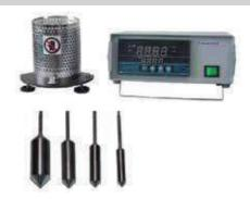
Thermosel for elevated temperature testing. The temperature can be used from environment temperature +10 °C to 250 °C. SC21, SC27, SC28, SC29, four spindles is configurated.
