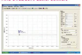
Viscometer can select Gather software to automate collect data, save data, compare many history curve. Data can be saved as a file or exported to excel format.
